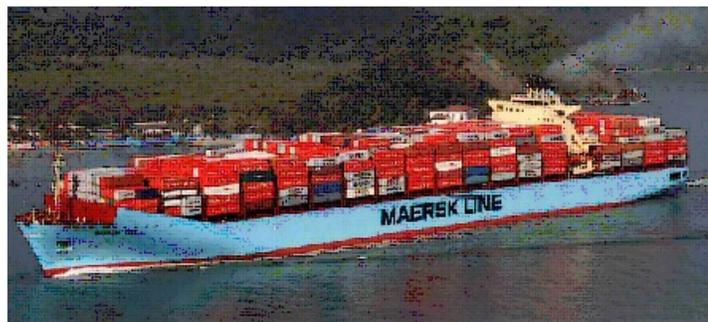
The Maersk Sammax class vessels have an overall length of 984 feet and a beam of 147 feet. The shape is optimized for operational efficiency; Maersk claims fuel efficiency 8% better than other ships of equivalent capacity.
